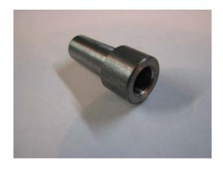
Can I still use my old UNIMAT accessories? Yes, you can. The new spindle comes with a M12-1.0 mm threaded end at the spindle head. Thus all screw-on type accessories can be used. In addition, LatheCity offers an adapter for using straight pin UNIMAT accessories such as life centers. That adapter is a Morse #0 taper to ~7.2 mm straight hole adapter. We do also offer Morse #0 blanks if you want to machine yourself Morse type gizmos.
